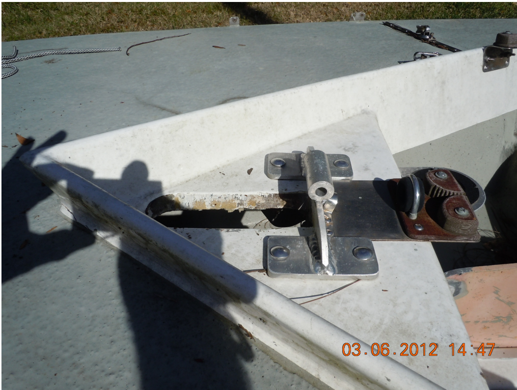
Permanent pivot mounted at mast opening. Doubles as vang purchase but could be demountable using recessed threaded fittings
