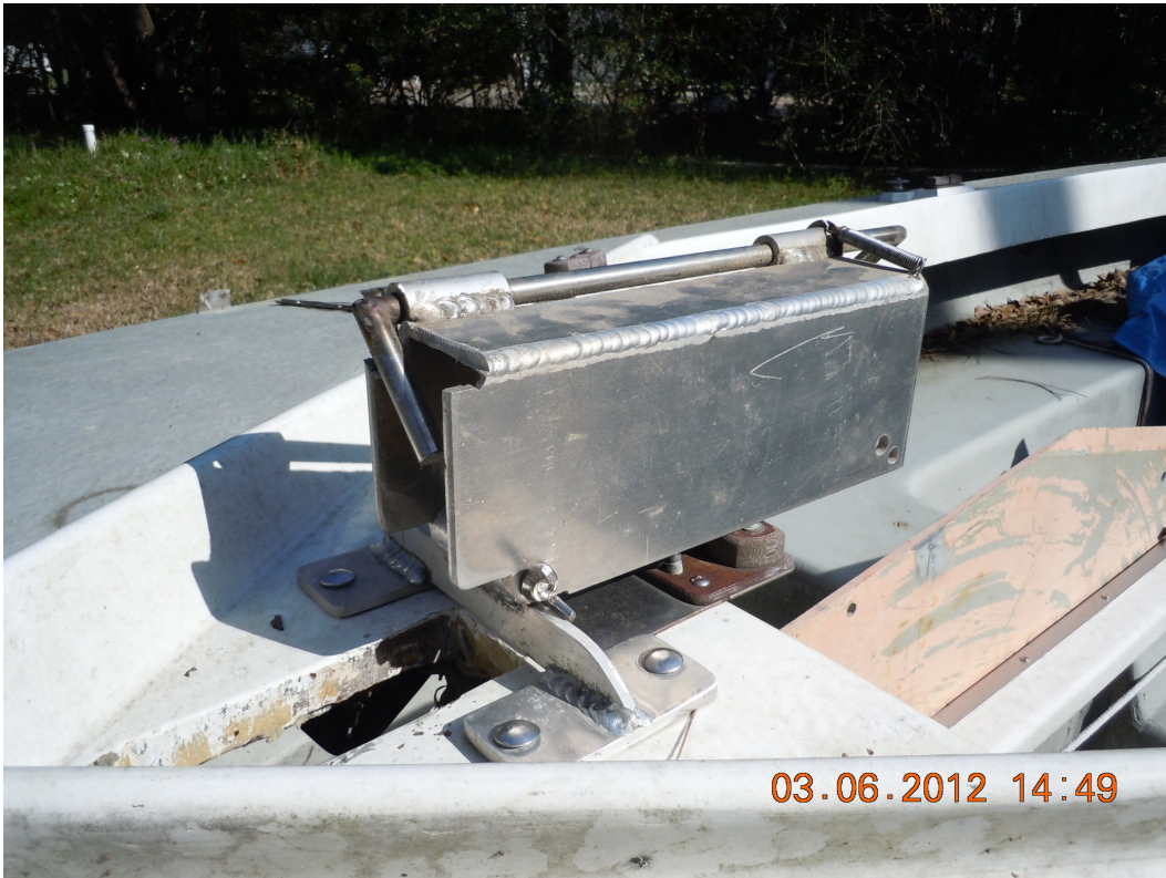
View with pivot bolt in place and ready to receive mast. Note stopper rod location.
