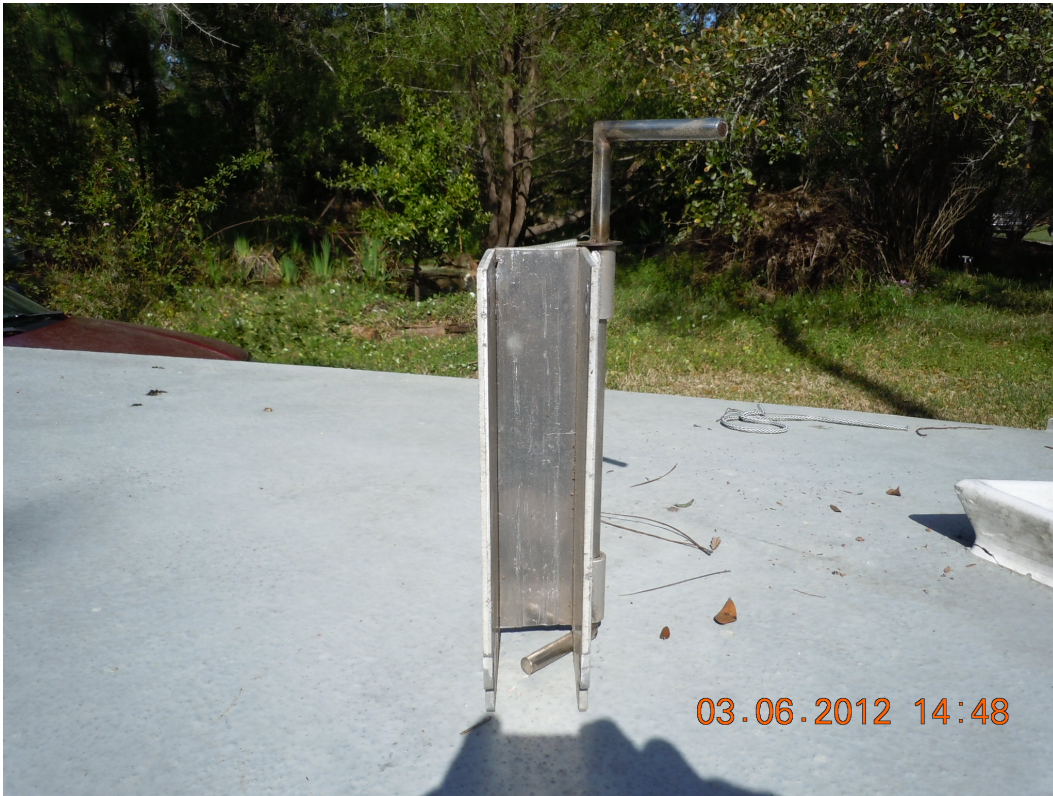
View of open end of housing. Note stopper rod at bottom.
