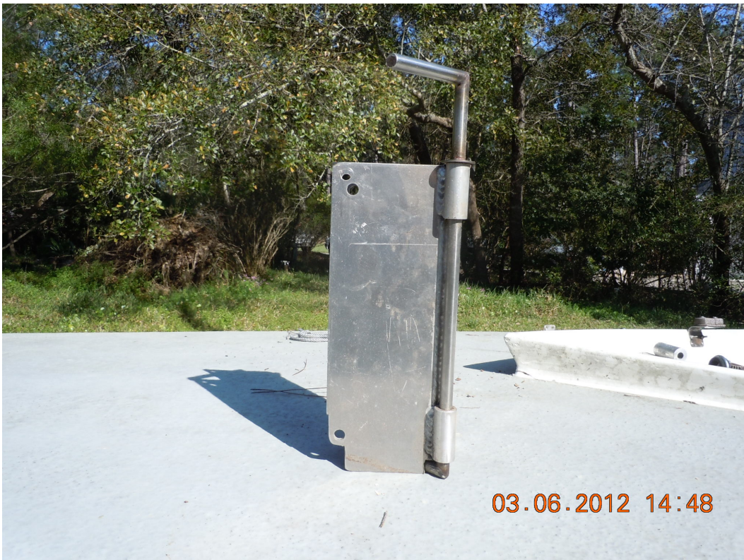
Side view of housing that captures bottom of mast. Stainless bar is spring loaded stop that keeps mast footed. Hole at bottom left fits to deck pivot, top left hole is for bolt that retains mast in housing.
