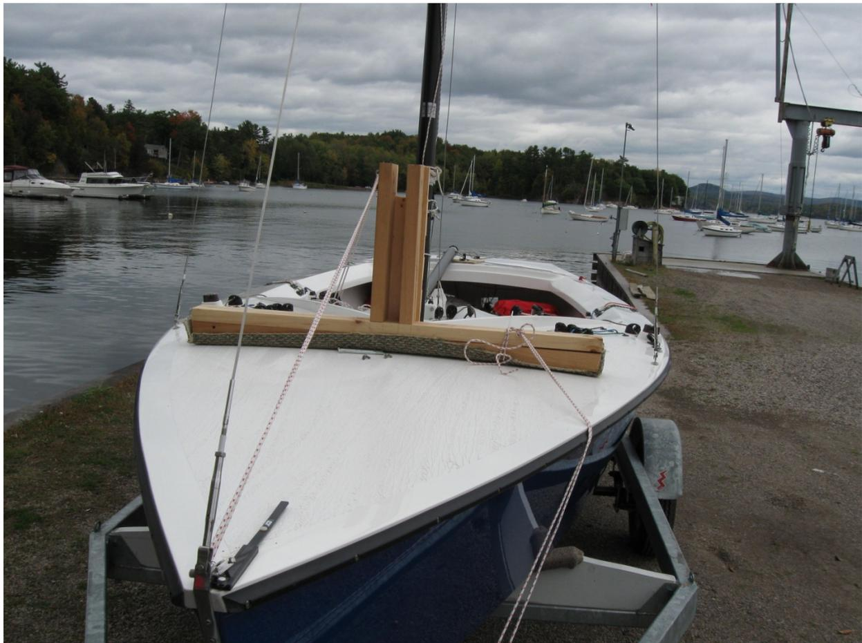
The next step is to make the gin pole itself. Mine is made from 2 pieces of 2 x 4 scarfed together to make a total length of 15 feet. I used fir lumber because it was available and lighter than standard pine. At the top of the gin pole I fashioned a "crane" to permit attachment of the 4 part block and tackle system. On the way to or from the launch site this pole is tied alongside the mast itself. See picture below:
